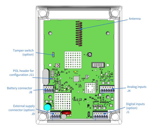
The analog and digital connections and the external supply are detailed in the corresponding chapters.
