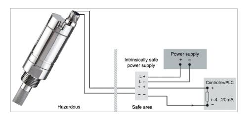
The FA 515 Ex measures dew point or pressure dew point in potentially explosive atmospheres and can be used in many nonaggressive gases.
