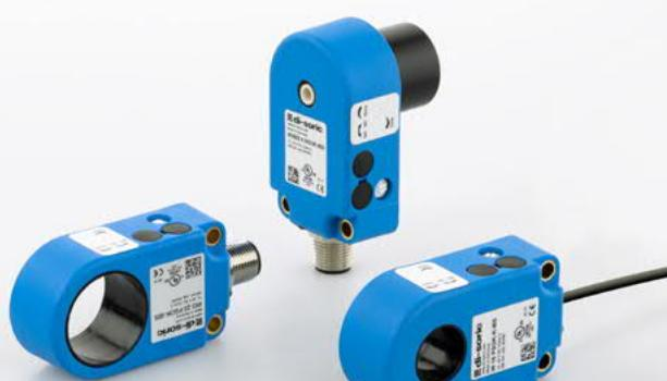
Our inductive ring and wire breakage sensors detect the smallest metallic parts that are conveyed in supply tubes for further processing. In the case of parts that are fed very quickly, the integrated pulse stretching generates an output signal that can be easily analyzed. All devices from di-soric are reliably protected against overload, short-circuit and polarity reversal.
