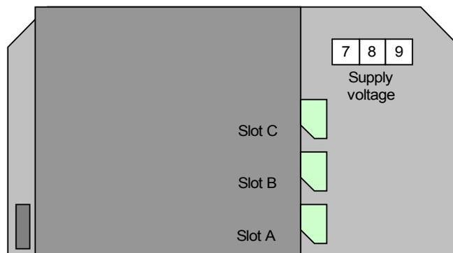
In the 24VDC model the power supply is connected in the base card terminals 7 and 9. The polarity does not matter. The connector is green.
