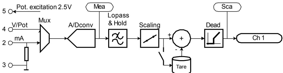
The microcontroller sets the multiplexer "Mux" to measure the V or mA input
