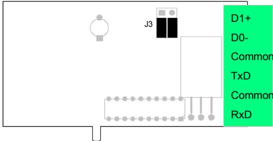
The serial communications card 2000-RS works most often with the factory set jumpers: no termination. But if the RS-485 bus is long (>50 m), the last device on the bus should be terminated.
