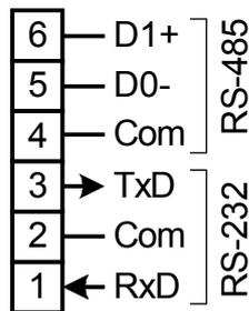
The RS-485 bus consists of two data lines and a common line. In the cable, the data lines should be a twisted pair. The more positive line at idle at terminal 6 is commonly called +, D1, A, or B. Correspondingly the negative line at terminal 5 is called -, D0, B, or A. The common wire is connected in terminal 4. The shield of the cable should be earthed at one point only.
