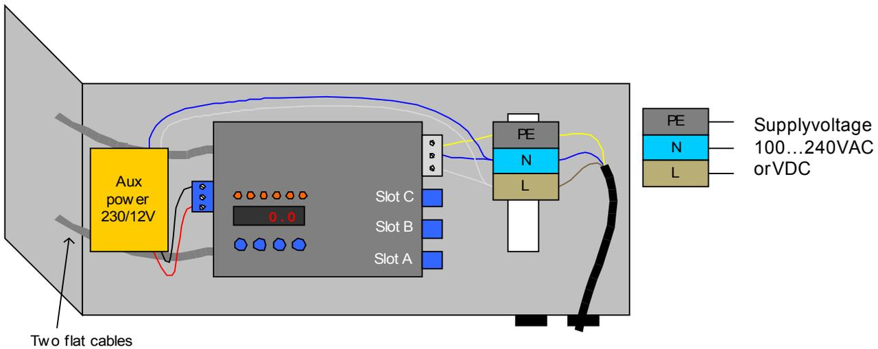
Bring the Live, Neutral, and Protective Earth wires to the connectors mounted on the DIN rail. The other power supply cabling is factory installed.
