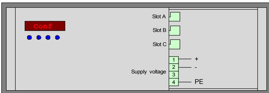
The power supply is brought to the lowest connector terminals 1 and 2. The polarity does not matter. The enclosure may be earthed using the terminal 4.
