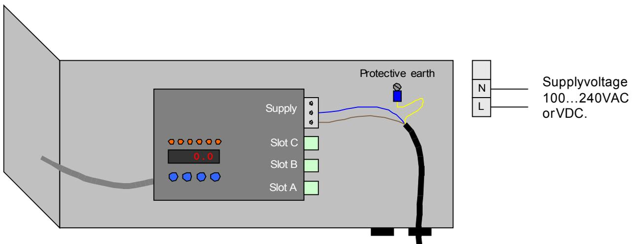
Bring the Live and Neutral wires to the electronics unit as in picture. Connect the Protective Earth wire to the M4 screw using the Faston connector provided - a Faston crimping tool is needed. A pre-fuse is not necessary, but if one is used, it should be at least 500mA.
