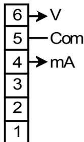
The analog output card provides one mA or V output signal. These can not be used at the same time.
