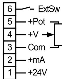
The potentiometer upper end is connected in terminal 5, feeding 2.5 V excitation. The lower end is connected in 3. The wiper is connected in terminal 4.
