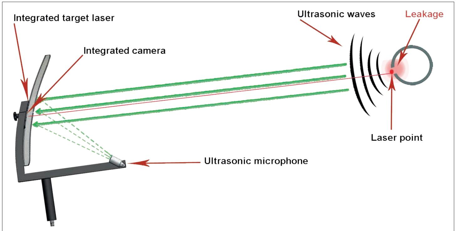
By bundling the ultrasonic waves in the parabolic mirror, even the smallest leaks of 0.8 l / min (ca. 8 € p.a.) at a distance of up to 10 ... 15 m can be localized with pinpoint accuracy ( $\pm 15$  cm). The shape of the parabolic mirror ensures that only ultrasonic waves of the targeted leak are evaluated. Noise is reduced to a minimum.
