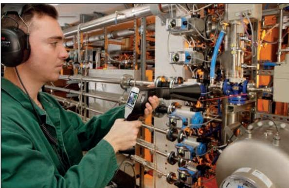
The noise-proof headset enables the leak detection also in EXTREMELY loud ambient. The ambient noise will be faded out, the leakage (inaudible ultrasonic sound) will be transformed to an audible signal. The laser grants an exact locating.
