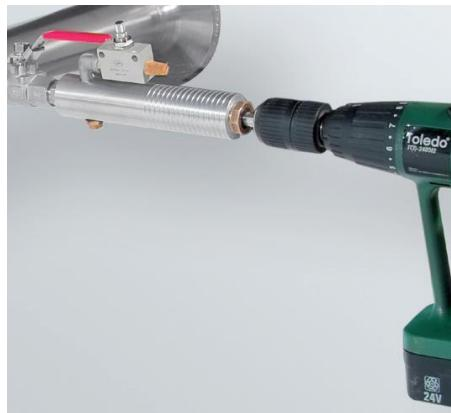
In case the system could not be shut down, means to be set depressurized, there could be used the CS spot drilling collar (Order-No. 0530 1108) and drilling jig (Order-No. 0530 1108) to drill through the ball valve.
